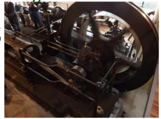
The Stott mill engine at the museum has been lovingly restored by our volunteers and will run on live steam for the first time this year, over the Bank Holiday Weekend. The engine has the power of 250 horses. The 10 foot flywheel is cast in iron and weighs 10 tons on its own.
